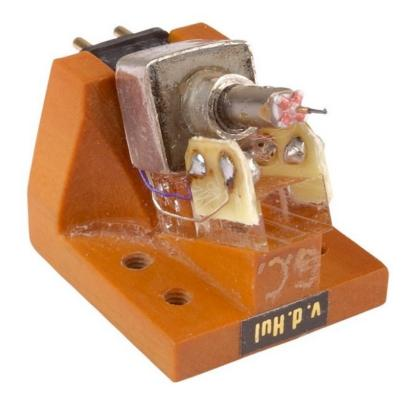
The coils at the front of the cantilever became shorter than usual
