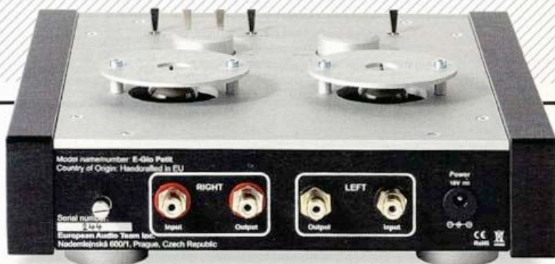
ABOVE: Simplicity itself – single gold-plated RCAs for connection to the tonearm leads and out to your choice of (pre) amplifier. Note \pm 18 V DC PSU input socket
