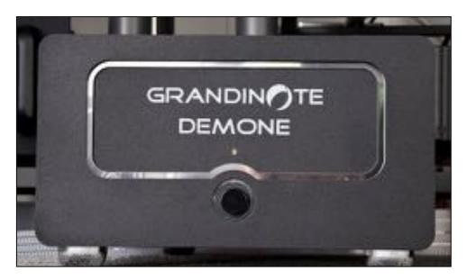
Demone provides 60W per channel (at 4 and 8 Ohm) with an impressive damping factor >230 and a highly extended frequency response (1,5Hz - 350 kHz).
