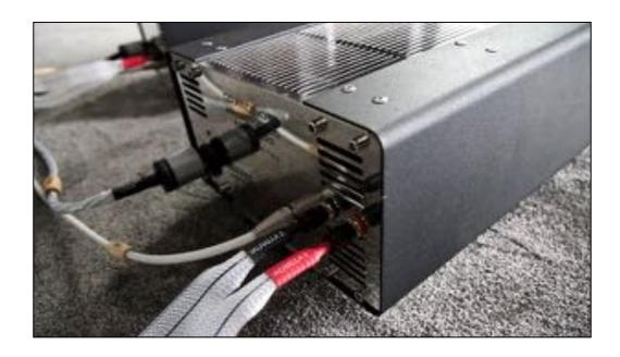
Each monoblock offer one fully balanced XLR input. All the circuits operate fully in Class A, with no feedback and direct coupling stages use no capacitors between stages. Each amp draws approximately 220W, which is not that much compared to some tube amps and due to the pure Class A operation amps can get quite hot, so a proper space around is needed to provide enough ventilation.
